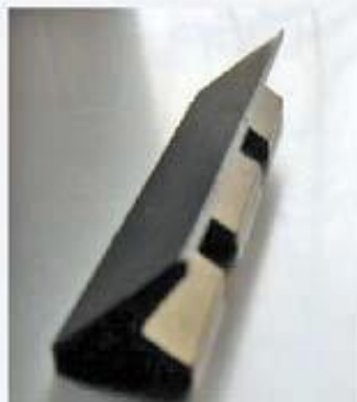
Scraper for hot oil removal from the shaft
