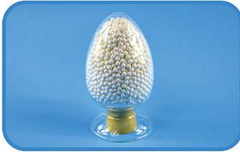
Activated Alumina as Hydrogen Peroxide Absorption
