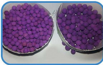
Potassium Permanganate Activated Alumina
